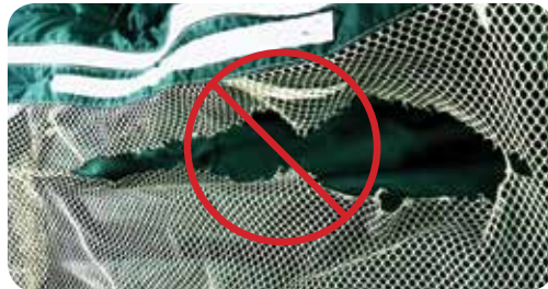
Canopy and netting have tears, holes, or abrasions.
